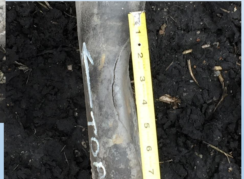
2-in by 1/16-in Crack
